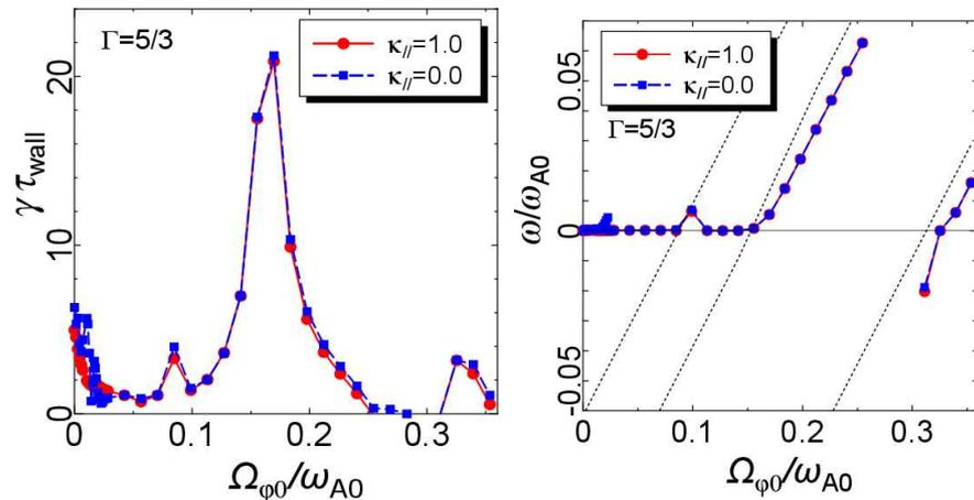
In the incompressible case, sound wave damping has no effect on stability (consistent with theory).
