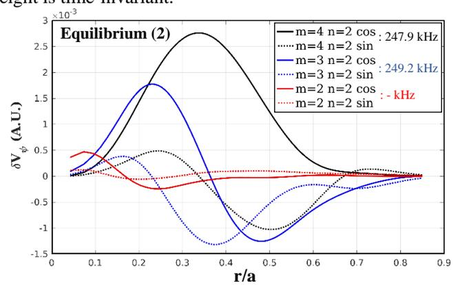
**Figure 2:** Spatial profile of radial velocity harmonic of  $n/m=2/3$  GAE in nested flux surface equilibrium.
