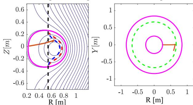
Fig. 1 (Left: Poloidal view) Dashed blue is UHRL, dashed red is R-cutoff, dashed black is ECR layer, (Right: Toroidal view) dashed green is magnetic axis
