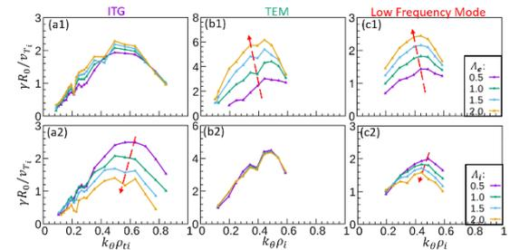
Fig. 2 linear growth rate spectrum of ITG mode (a), TEM (b) and low frequency mode (c) when  $A_s$  is changed from 0.5 to 20 respectively.
